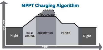
Figure (12.1) Charge controller curve
