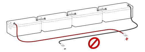
Figure (2.2) Incorrect battery polarity
