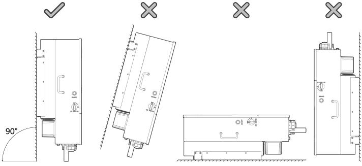
Figure (1.3) Inverter position
