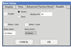
Figure (9.3) Parallel setup
