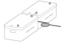
Figure (4.2) Temperature Sensor
