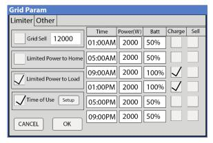
**Charge**: Allows the batteries to charge from an external AC power source, such as a generator or grid, during the hours selected, up to the voltage or % configured. If the external AC power source is a generator, it is also necessary to meet the condition "Start V" or "Start %" located in the Battery Setup to begin charging from a generator. The PV array will charge the batteries at 100% regardless of the "Charge" box in TOU. Do NOT enable "Charge" and "Sell" at the same time.
