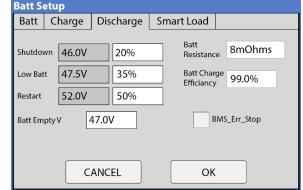
Low Batt: Low battery voltage (battery symbol on the home screen will turn yellow). Stopping point for TOU.
