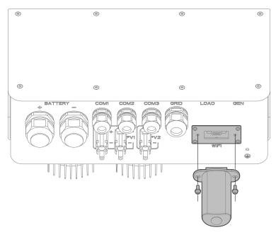
Figure (7.3) Plug in the dongle
