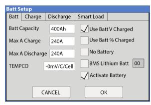
Figure (9.5) Battery setup
