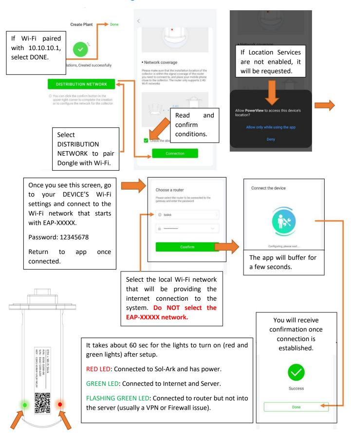
Figure (7.14) Wi-Fi dongle lights
