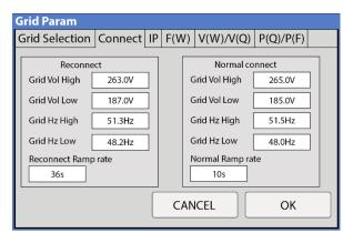
Figure (11.6) Voltage /Frequency range
