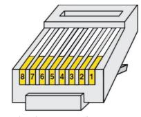
Figure (13.4) RJ45 port configuration.
