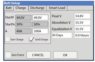
Figure (3.2) Battery charge settings
